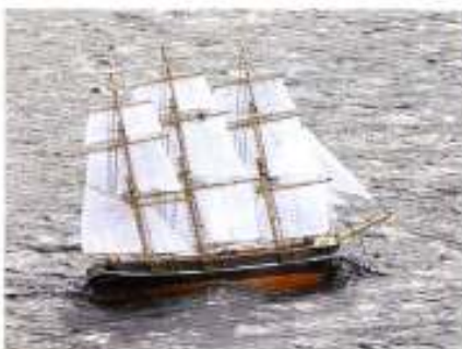
ABOVE: With five sails removed, beating on a very windy day. If the sails are caught aback in these conditions, there will be a sharp stop, and violent change of direction
