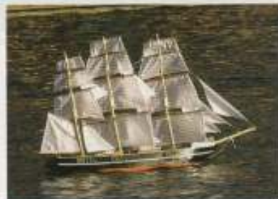
ABOVE: The little full rigger (square sails on all masts) as described in the schematic. She is sailing 'hands off' in a good beam wind
