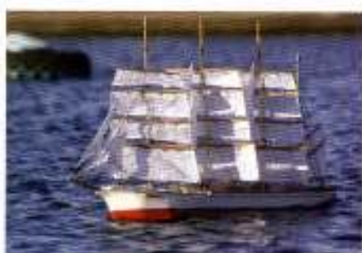
ABOVE: Sometimes it all goes wrong! The strong wind has just gone round 180 deg, and what was good progress beating on the starboard tack, has turned into sails all aback with the wind from ahead. The model is now about to go astern until use of the rudder makes her head fall off the wind, so that control can be regained
