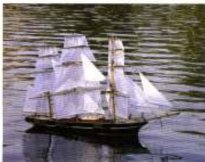
ABOVE: Going about from starboard to port tack. The bows are being pushed round by the backed foremast sails
