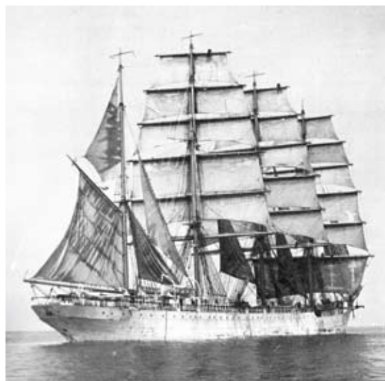
ABOVE: 'Viking', a very powerful, four masted barque. Note the sailors on the main and mizzen royal yards
