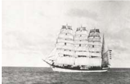
ABOVE: Typical of late 19th Century, large square-riggers, the 'Lord Ripon'. Note the skysails on each square-rigged mast
