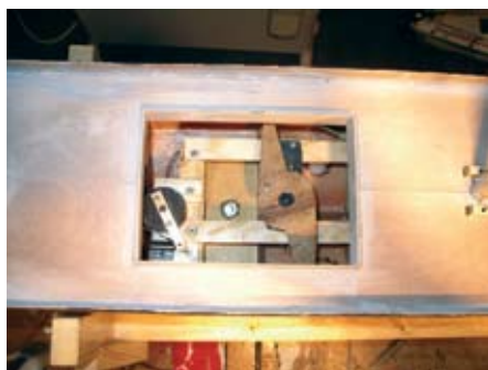
The 'false deck' between the fore and main masts, with the small servo for the outer jibs, and the sail arm servo for the foreyards, seen below deck. The large bolt head in the centre of the picture is one of the locating bolts for the detachable sailing keel
