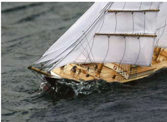
This is why sailing ships had flared bows! The deeper she drives into a head sea, the more buoyancy she has, and the better her chances of rising to it
