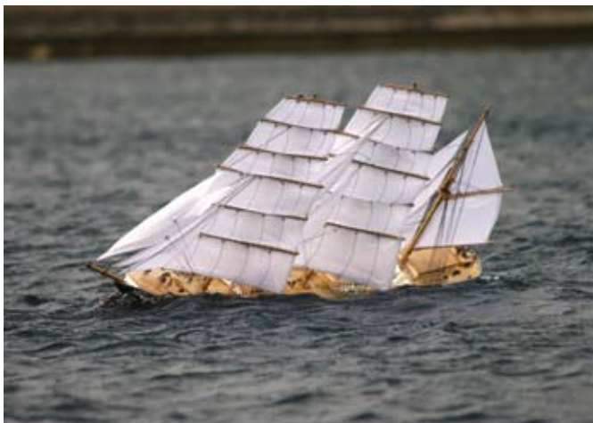
This is 25 mph of wind, and, even with a 7 kg keel, she has as much wind as she can stand, without reducing sail. Even in these conditions, she can be tacked with assurance
