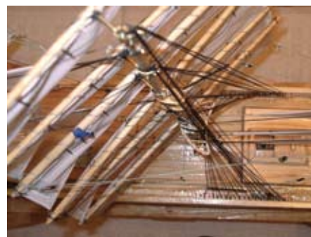
Looking down from above the main mast, with the shrouds and backstays fanning out from the mast to the bulwarks. In this picture, the yards are not braced fully round, on to the backstays, they will go further, and will need to do so to sail close to the wind
